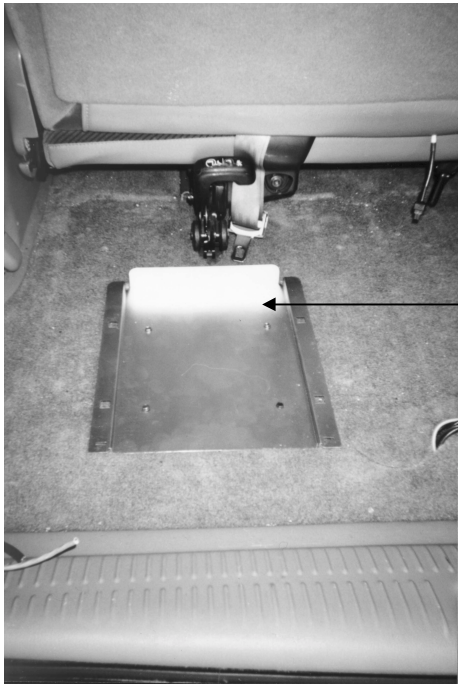
Figure 38 Navigator Base Plate in Position
