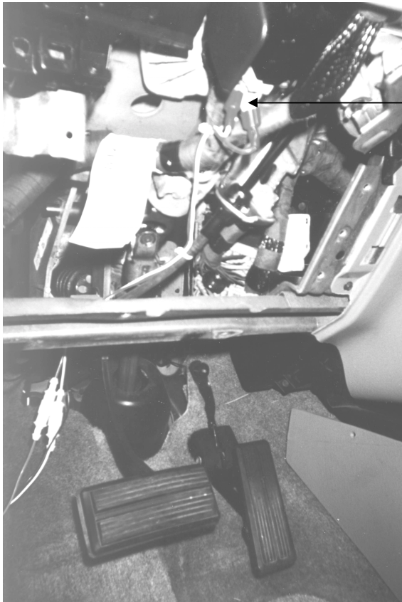
Figure 40 Ignition Sense Lead Connected to the Vehicle
